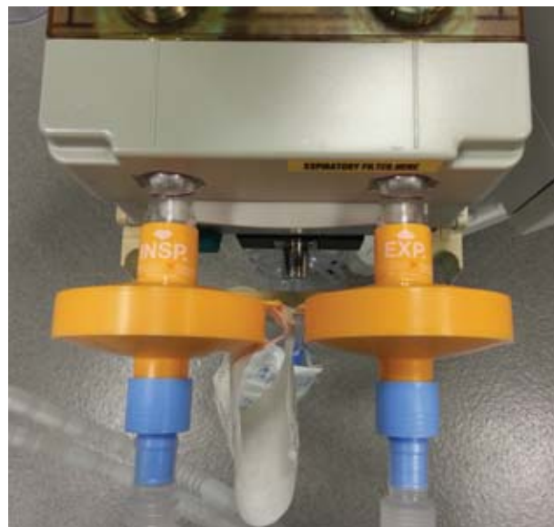
Figure 3. Placement of activated charcoal filters at the inspiratory and expiratory ports can help remove traces of the triggering anesthetic gas.
